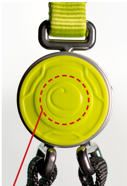
Example of an embossed plastic shell on a defect-free lanyard that we have already checked
